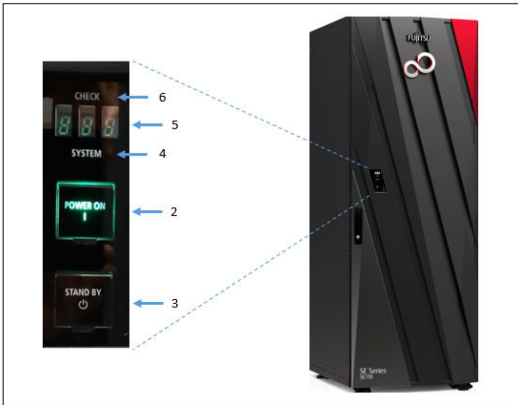
Figure 13: Control panel on the rack of the SE710
