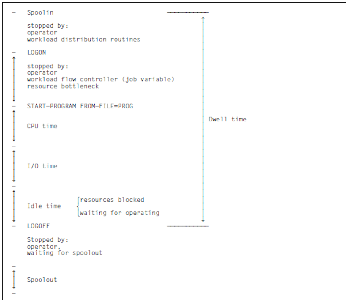
Figure 2: Time definitions in batch processing
