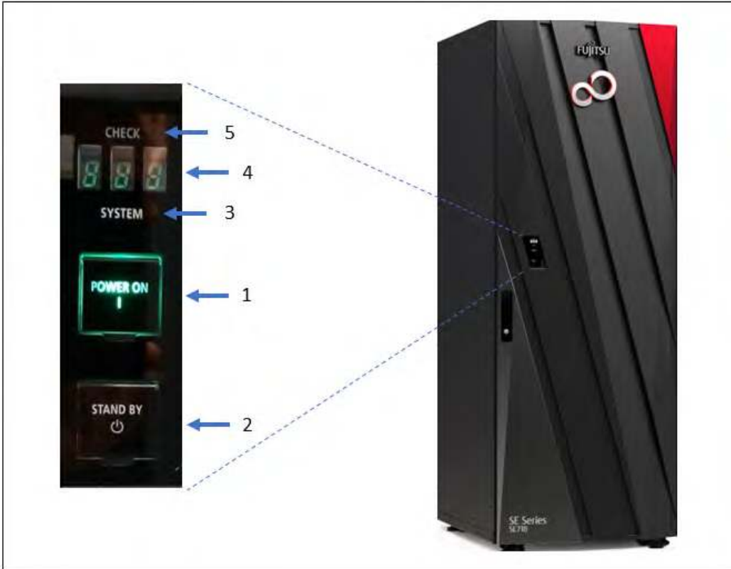
Figure 7: Control panel on the rack of the SE710/SE730
