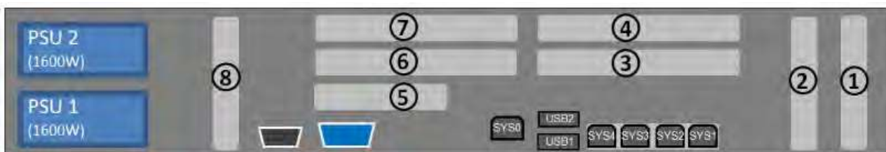
Figure 7: AU47 M5 - principle of PCIe slot assignment at the rear of the device
