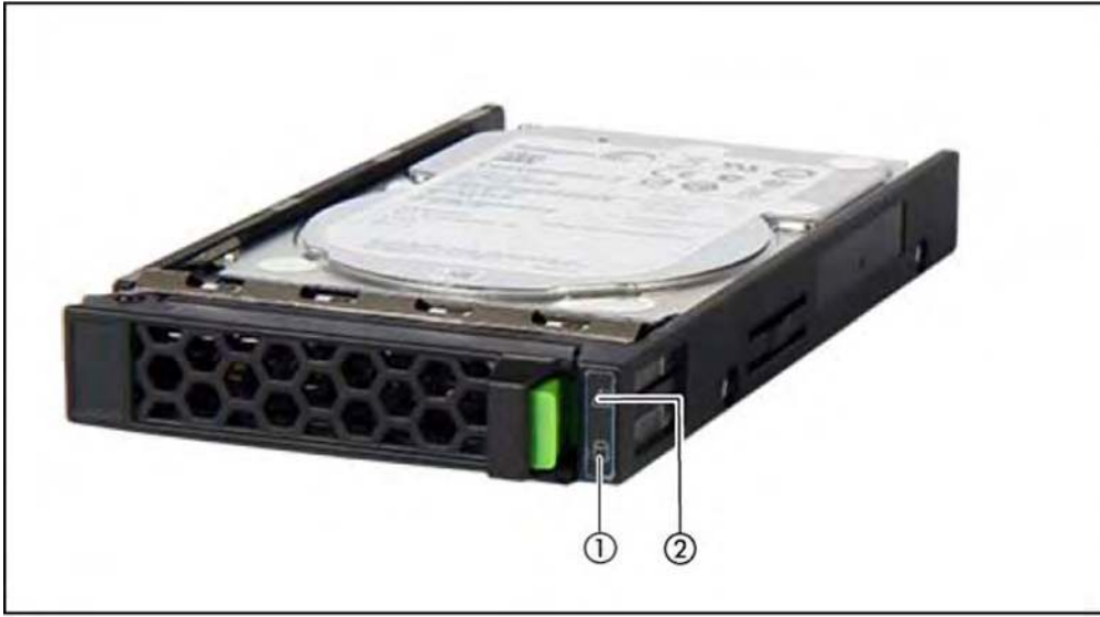
Figure 5: Indicators on a hot-plug HDD module
