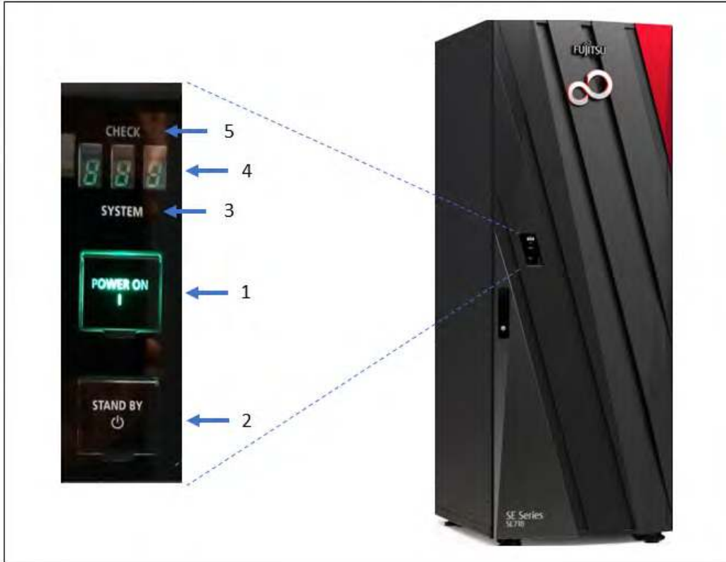
Figure 7: Control panel on the rack of the SE710/SE730/SE730B
