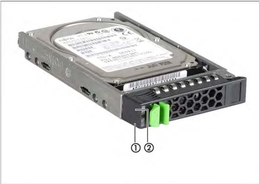
Figure 13: Front - Detailed view: Indicators on a hard disk module
