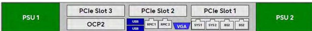
Figure 48: HNC M5 (SE730B) - principle of PCIe slot assignment at the rear of the device
