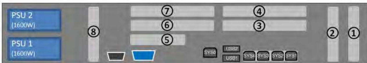
Figure 14: Principle of PCIe slot assignment at the rear of the device (SU310)
