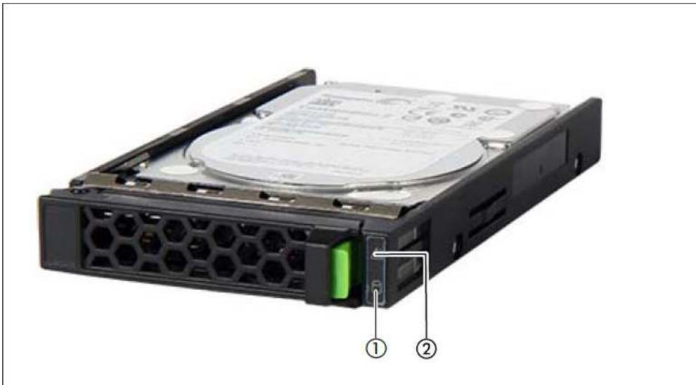
Figure 13: Front - Detailed view: Indicators on a hard disk module
