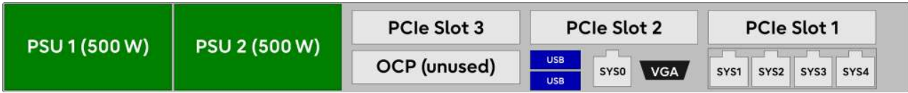
Figure 46: HNC M4 (SE730) - principle of PCIe slot assignment at the rear of the device
