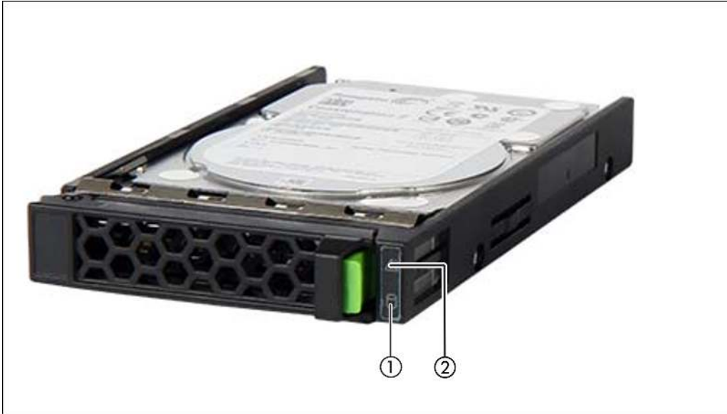
Figure 7: Indicators on a hot-plug HDD module
